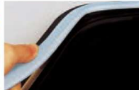
Channel Installation 1. Apply an adhesive silicone between the channel base on fixture housing to prevent slippage and stretching over time 2. Press LED Flex Tube into the channel with even pressure from the beginning to the end.
