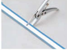
Cutting Mark Must be cut only on the indicated mark
