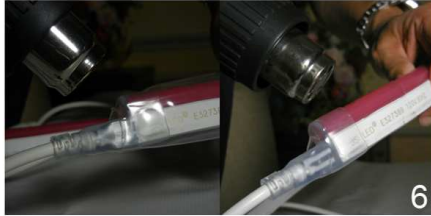
Heat both side of the shrink tube with a heat gun on
